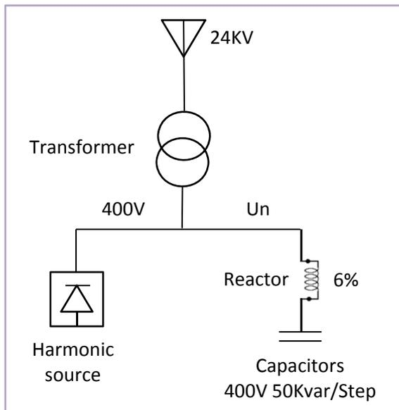
If you bring 6% reactor connected to capacitor in series and require reactive power of each step equal to 50 kVAR at 400V, you can calculate  $U_1$  and  $Q_1$  as follows:
